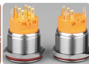
镀金/银插脚/银触点 Silver/Gold Pins/Contact
