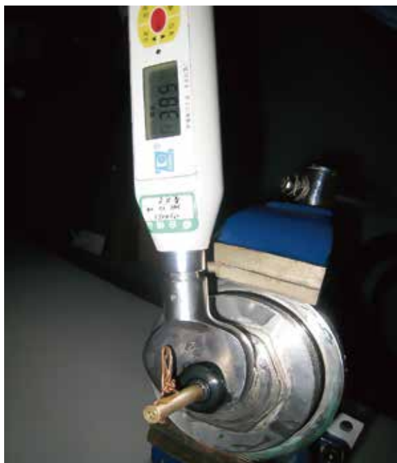
电缆接头夹紧扭矩测试 Torque moment test according to EN50262
